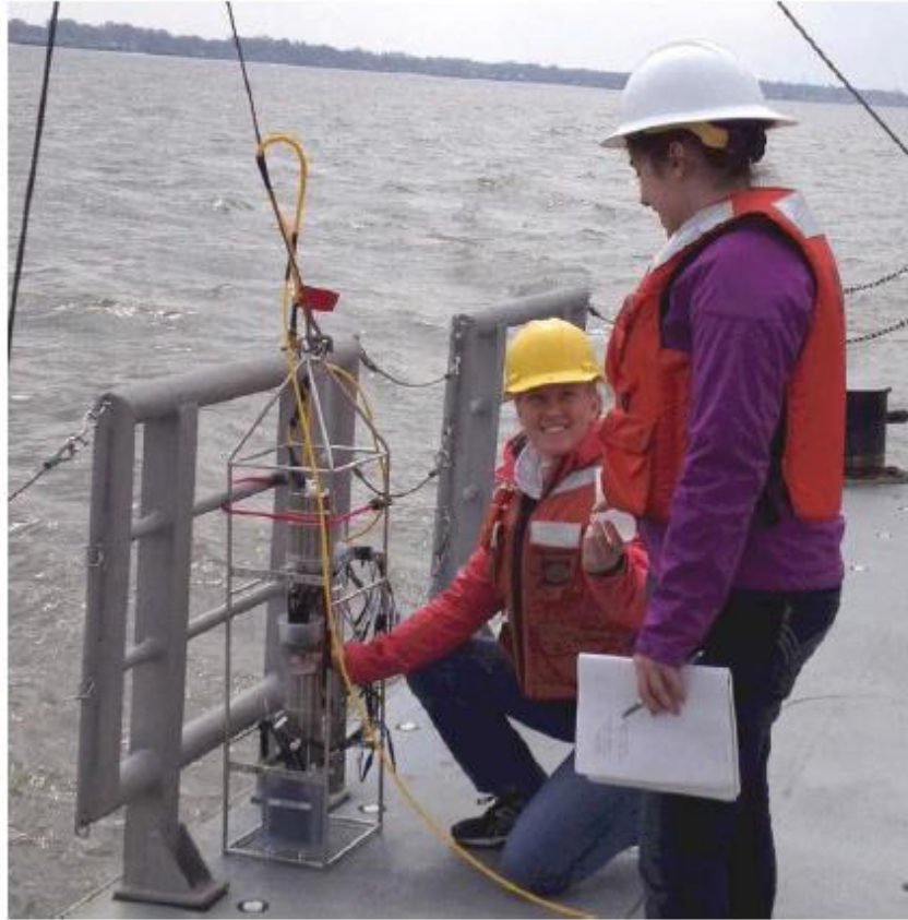
Figure 7. Two Tufts University students calibrating sensor array prior to being deployed.
