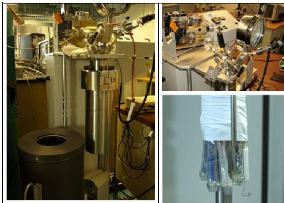
Figure 2. The custom built high pressure/temperature chamber for testing the ISE sensors (left). High pressure reagent injector system (top right) and the ISE sensor array (bottom left)
